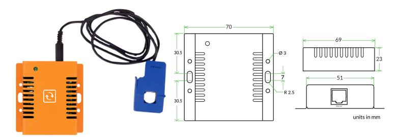
Non-intrusive plug & play current sensor. This sensor allows you to assess the state of legacy equipment by analyzing its current (power) usage. It seamlessly integrates with SNMP and Modbus TCP, enhancing your monitoring systems. Determine an equipment's operational status and performance effortlessly by placing the clamp around the power cable and initiating monitoring. Specifically designed for equipment with a power rating of up to 100A.
