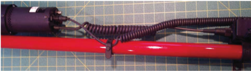
Picture 1: Fasten the axial cable lead to the pole using the rubber strap provided. Note that the actual cable has longer axial lead than pictured to provide for swivel movement of test head
